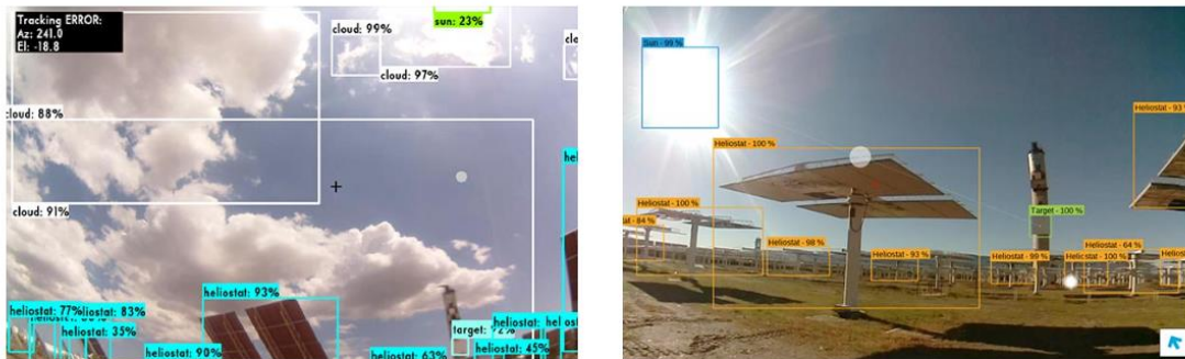
Augmented reality images processed on a mobile device at CESA solar field at CIEMAT-PSA.
