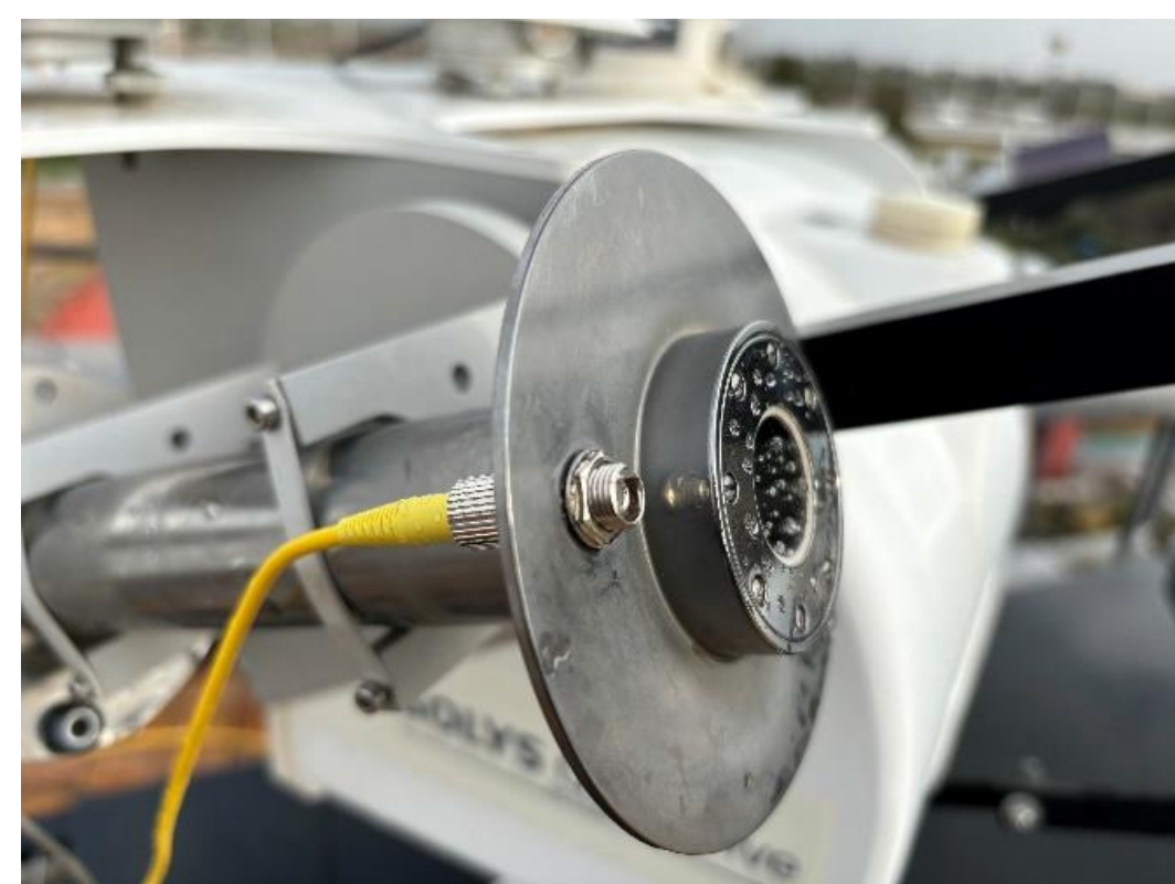
Optical fiber tip alongside commercial pyrheliometer.
