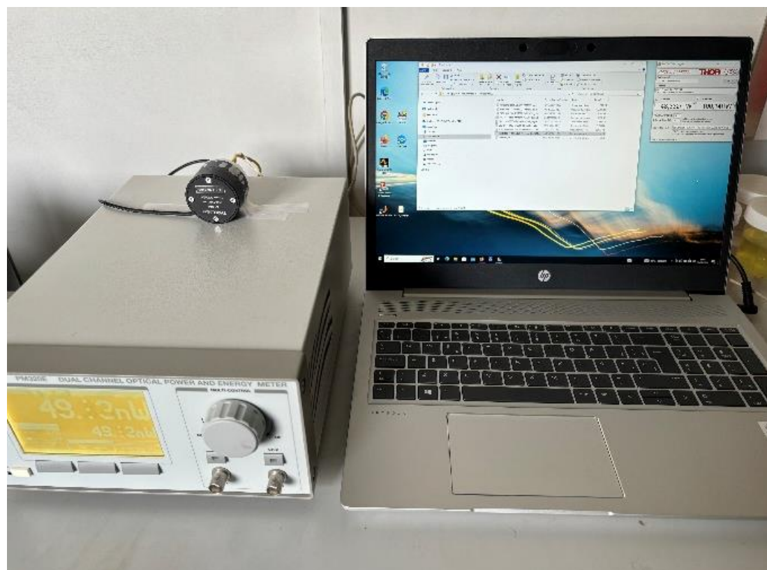
Photodiode, optical power meter and computer to store power traces.
