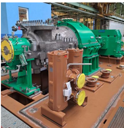
The Doosan's steam turbine with the gearbox (right), assembled turbine (left), and the oil frame (depicted in brown). A very similar high-pressure (HP) air turbine will be developed for ASTERix-CAESar project.
