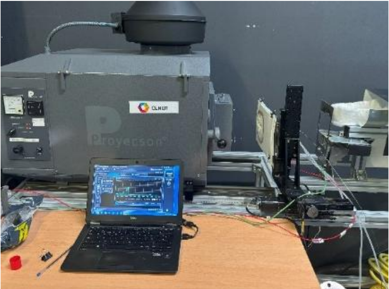
CENER's high-flux solar simulator
