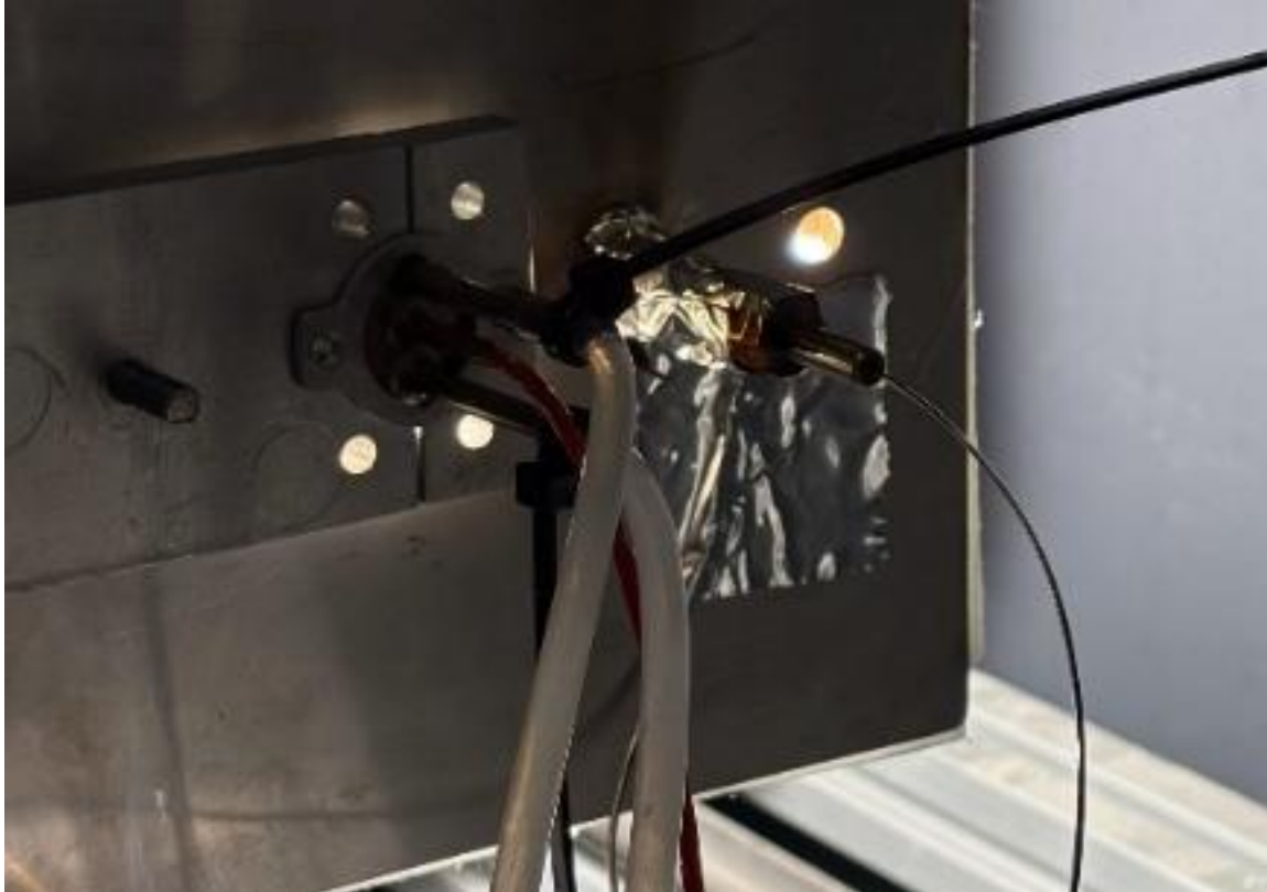
Front (left) and rear (right) of the steel plate used as mounting for the optical fiber, radiometer and thermocouple
