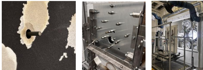
Fig. 1: (Left) Frontside of the Inconel steel plate, with one fiber tip sticking out of the plate; (center) Backside of the Incoloy steel plate, with two optical fibers embedded in the lower part; (right) High Flux Solar Simulator KIRAN-42 (IMDEA Energy, Móstoles, Spain) with the central lamp on.
