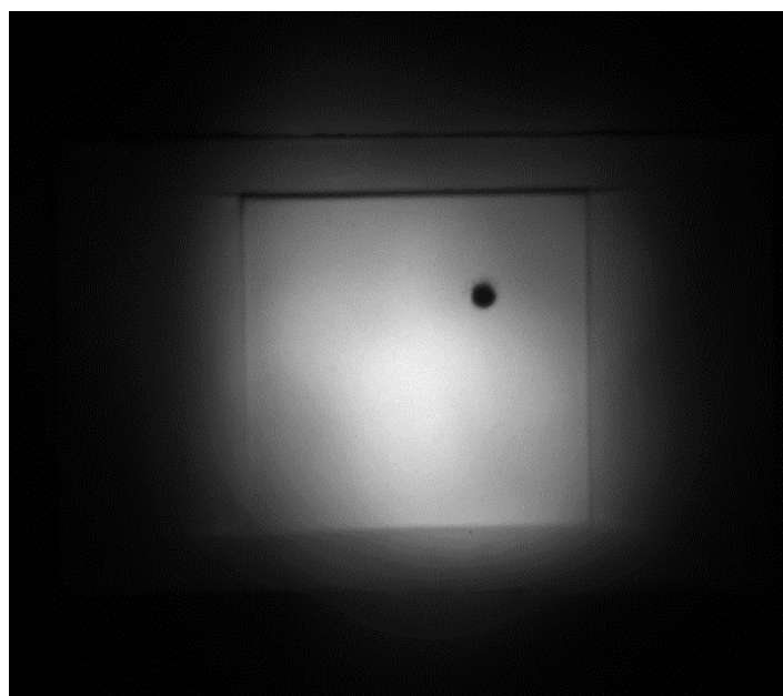
Figure 5: Target installed at the tower for performing the aiming strategy tests and a Gardon sensor (black circle) to measure the flux and compare with simulations.
