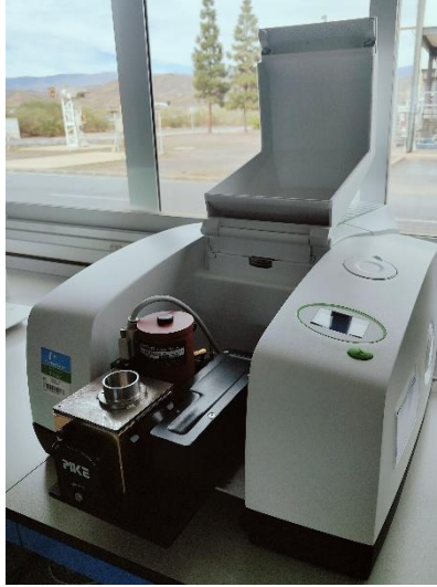
Figure 11: Perkin Elmer Frontier FT-IR spectrophotometer used for infrared reflectance measurements
