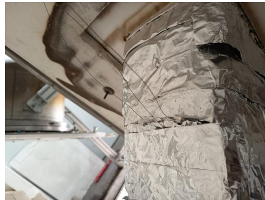
Figure 35: Latest 20 PPI SiSiC foam installed and being tested at IMDEA (left); 3 additional thermocouples installed (right)
