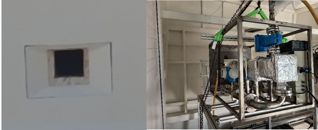
Figure 20. a) Pyramidal thermal shield and b) structure for skid positioning
