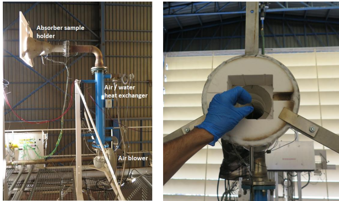
Figure 8: Solar furnace thermal air loop (sample holder, air water heat exchanger and air blower)
