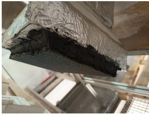
Figure 35: Latest 20 PPI SiSiC foam installed and being tested at IMDEA (left); 3 additional thermocouples installed (right)
